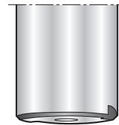
The front leading edge can be used for optical presetting.
