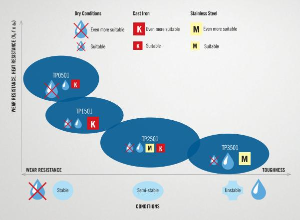
The grade chain provides a very versatile and comprehensive range to cover the whole steel turning area. TP2501 is the most versatile option, while TP3501 is the most secure choice. TP1501 provides competent performance and balanced productivity for applications in low-alloy steels or using lower speeds. TP0501 offers a high-heat profile in general steel machining, particularly in high-alloy steels.
