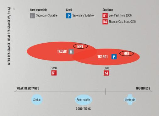
TK1501 is the first choice in ductile cast iron. TK0501 is the first choice in the grey cast iron area. TK0501 also works well in continuous applications in ductile cast irons. TK1501 can be a better choice at limited speeds with better toughness in demanding grey cast iron applications.
