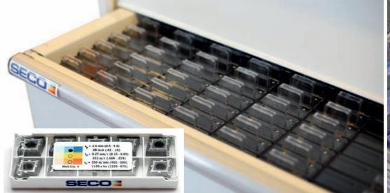
Inserts should be stored in such a way that the needed insert can be quickly retrieved.
