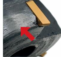
Immediately replace damaged tool holders and spare parts.
