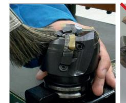
Pair the correct cutting edges with the correct toolholders. Inserts must be clamped in clean and undamaged insert pockets.
