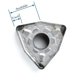
Use the appropriate insert dimensions for the operation.
