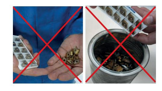
Cutting edges are brittle. Ensure that they are not damaged by improper storage.
