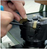
First position the insert correct in the insert pocket and only then clamp firmly.
